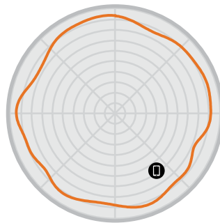
Figure 2. 5GHz Azimuth Antenna Patterns
